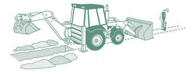
By hand, dig trial holes to locate the exact position of all cables. Always use a spade or shovel – never use a pick, fork or power tool – push the spade or shovel into the ground applying foot pressure.
